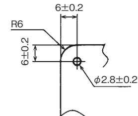
適応板厚 / Applicable panel thickness : =1.6
