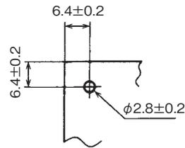
適応板厚 / Applicable panel thickness : =1.6
