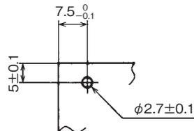
適応板厚 / Applicable panel thickness : =1.6
