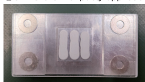
③CPVG thermal putty application
