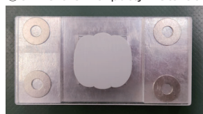
③CPVG thermal putty installation
