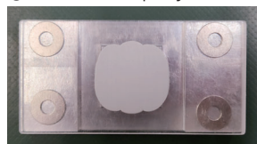
③CPVG thermal putty installation
